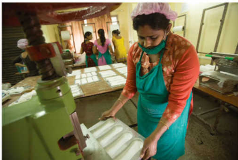
Aakar provides the raw material and distributes the finished product. Here, pine fibre is being pulverised and stacked in moulds before it is pressed manually
